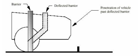
This type of collision is called an inelastic collision, where the momentum (p) of the vehicle equals the momentum gained by the bollard, as shown in the following equation. p = mv
